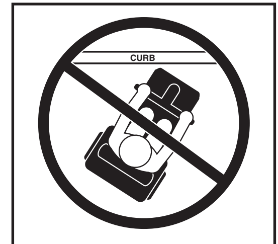
Figure 7. Incorrect Curb Approach
