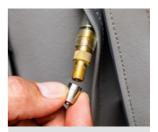
Ensure that the valve is tight and secure - then replace and tighten cap.
