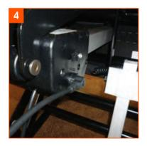
Connect the new handset plug into control box.
