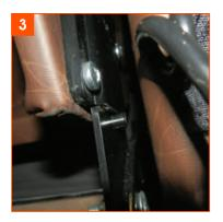
Carefully push the backrest down into place until the backrest bracket hits the stopper on the mechanism bracket taking care to make sure the backrest remains square and upright.
