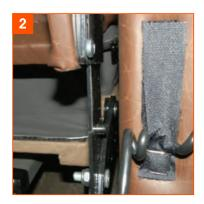
Insert one side of the backrest at a time, taking care to make sure the backrest remains square and upright.
