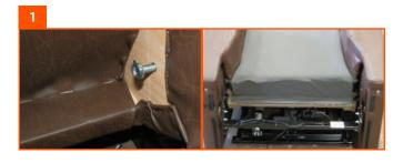
Remove backrest - remember to remove the screws securing the backrest brackets on the inside of the backrest
