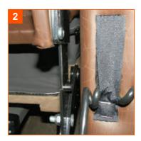
Loosen backrest brackets by applying upward pressure to the wings of the chair.
