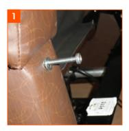
Using a cross-headed screwdriver, remove the screw from the back of the armrest.
