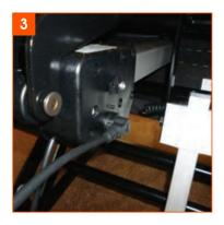
Disconnect the handset plug from the control box.
