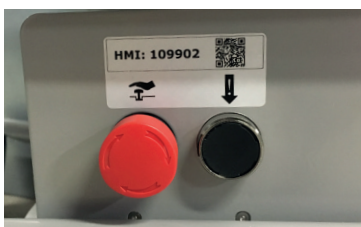
Emergency stop and lowering
