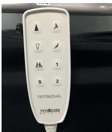
New hand control with more functions, for example two programmable memory buttons and one for safe transportation
