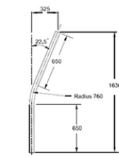
22.5° Bend Track – standard part dimensions
