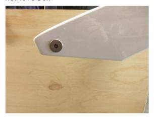
2. Insert Lifting hanger as shown and re-install bolt
