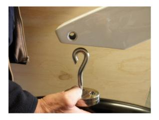
3. Tighten bolt with 2 x 6mm allen key
