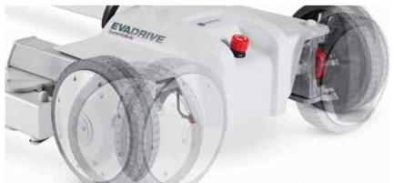
The rear wheels turn to any angle by using the control panel buttons.
