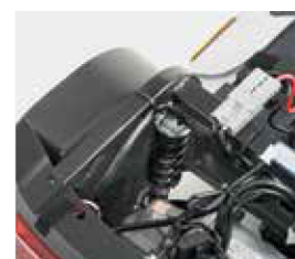
A fully suspended chassis provides a comfortable ride at all times
