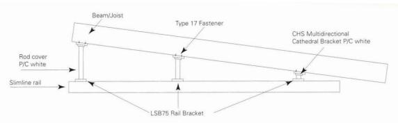
All exposed rod droppers and braces to be installed with AMS white rod covers for pleasing appearance.
