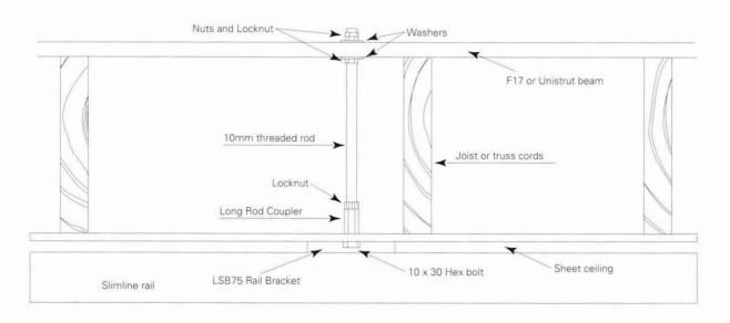
Where possible F17 / Unistrut beams should be staggered to spread load over 4 joists/ truss cords.
