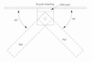
Rails may be installed at any angle exceeding 45° from wall surface.
