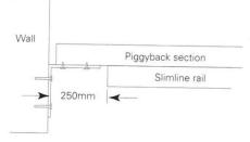
Spans requiring piggyback section should stop Slimline rail short at one end by 250mm to allow easy hoist/trolley removal for servicing.
