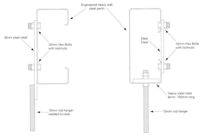
Suspension from steel perlins for Slimline and Fineline rail system may be made using normal suspension and brace methods. The integrity of perlins when loaded to required SWL of hoist system should be confirmed by a qualified engineer. Total deflections while under max. SWL should not exceed requirements of the standard AS/ISO 10535 2006.
